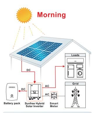
Optimized self-consumption will be achieved. Batteries are used to store the surplus energy generated by solar panels.
