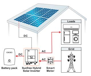
If the battery capacity is insufficient for self-use, electricity will be supplied from the grid.
