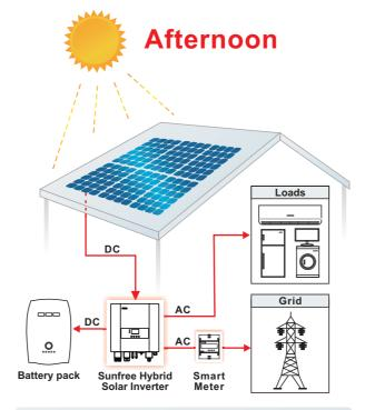
Surplus energy will be exported into the grid when batteries are fully charged and system self-consumption has been achieved
